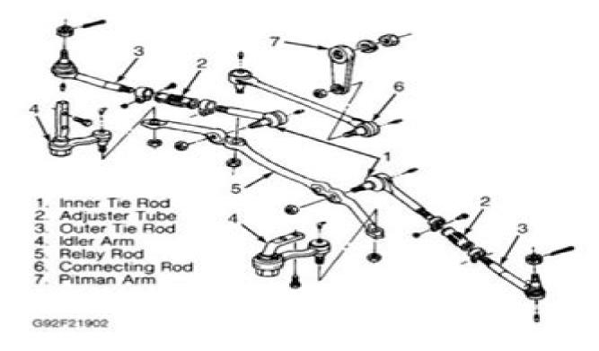
Fig. 2: Exploded View Of Steering Linkage (Astro & Safari - 2WD)
